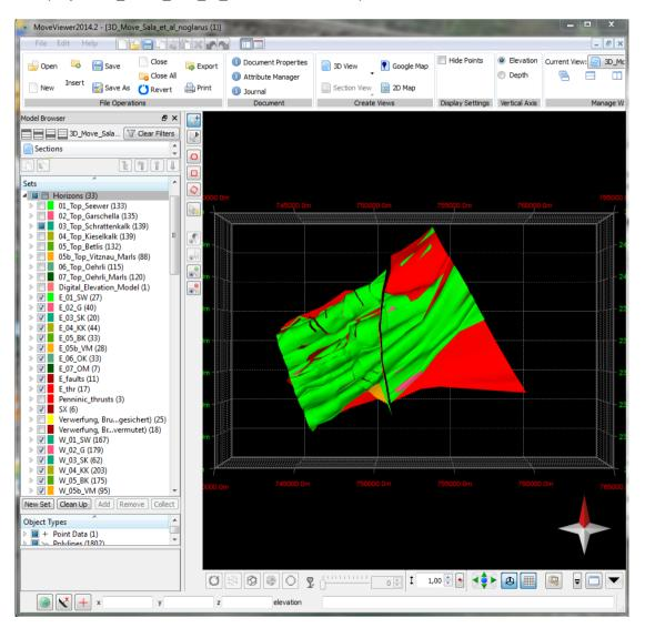
5) The surfaces are stored in the Model Browser (tree panel on the left side of the window), under "Sets". Scroll down until you can find the "Horizons" subset.
