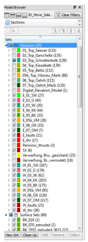
7) The surfaces are listed with abbreviations and are also divided in western and eastern surfaces (look for the prefix W and E). The items with a number prefix are the horizon lines from the cross sections.
